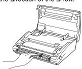
5. Gently wipe the white roller and the scanning glass surface with fax cleaning wipes, available at your local RadioShack store.
